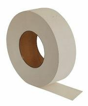
GSA Paper Tape is designed to strengthen joints when embedded in the first coat of the jointing system. 50mm wide Paper Tape is creased along the centre line to provide a crisp finish for corners and improved performance in automatic taping tools.
