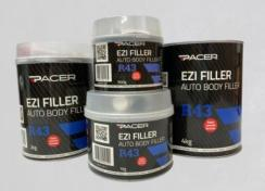
Pacer EZI Filler is a two-part, super smooth multi-purpose filler suitable for all autobody repairs with excellent adhesion to aluminium, fibreglass, masonry and wood surfaces. It cures in minutes providing an easy to sand, touch repair that can be drilled or tapped if required.
